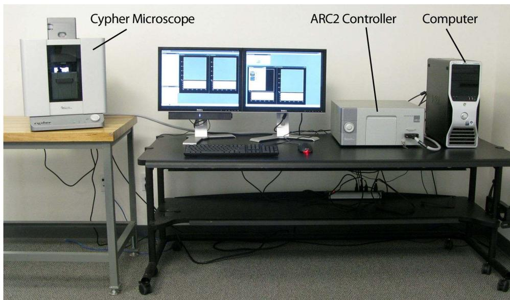
**Figure 1.1.:** Ideally the Cypher SPM is set up as shown, with the controller and computer on one table and the microscope on its own table. The air temperature controller (ATC) is not shown here. Please see [Chapter 19 on page 203](#) for more information.
