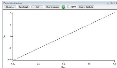
**Note** The 500M Ohm resistor should allow 2nA of current to flow for 1V of bias voltage.
