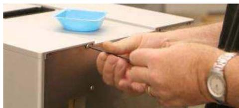
8. Replace the bridge in the front top of the enclosure. Slide it in so the screw holes and foam line up.
