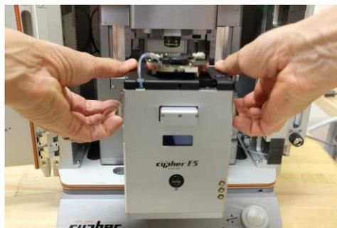
7. **Secure the scanner connector:**
