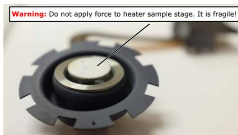
**Warning:** Do not apply force to heater sample stage. It is fragile!
