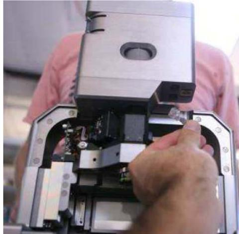
2. Remove the FireWire cable from the bottom side of the view module (black cable-like USB).
