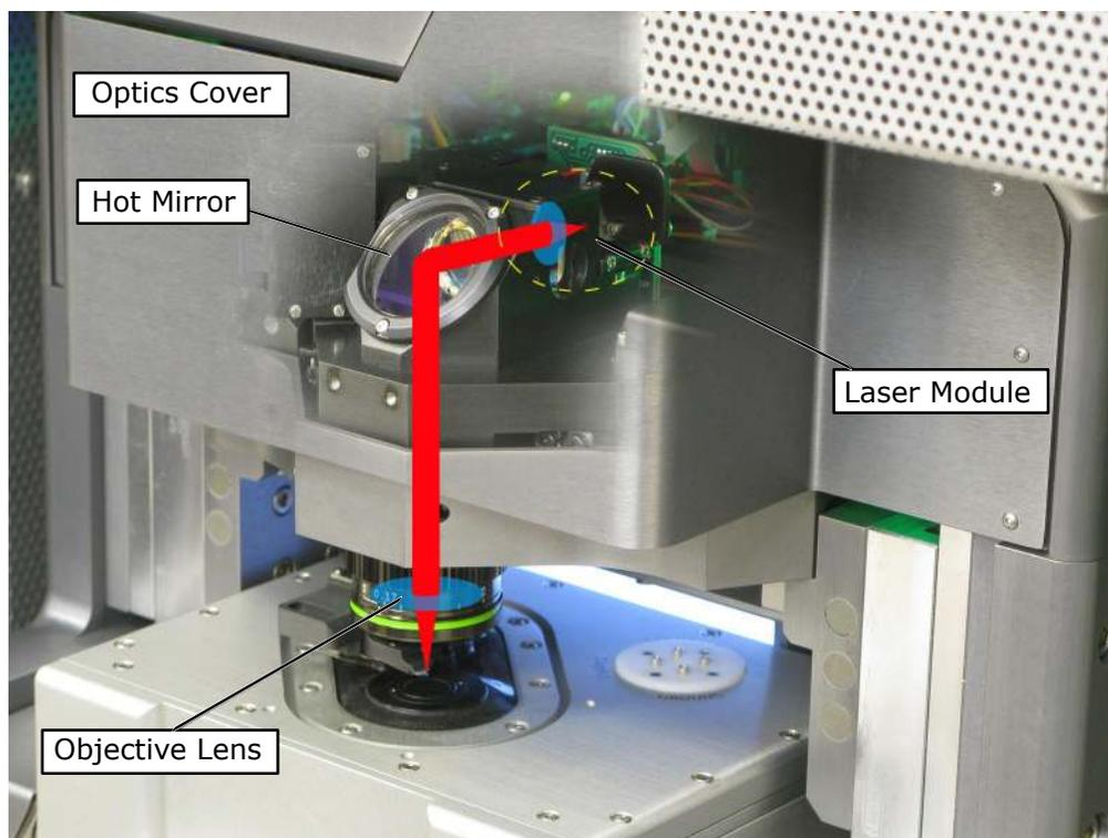
**Figure 20.3.:** Simplified laser path. Removing the optics cover exposes the hot mirror and laser module. The non-visible laser light originates in the laser module and comes out as a collimated beam. The collimated beam is reflected off of the hot mirror and into the objective lens, which focuses it onto the cantilever. During normal operation the only place a person can be exposed to the light is where the light exits the objective.
