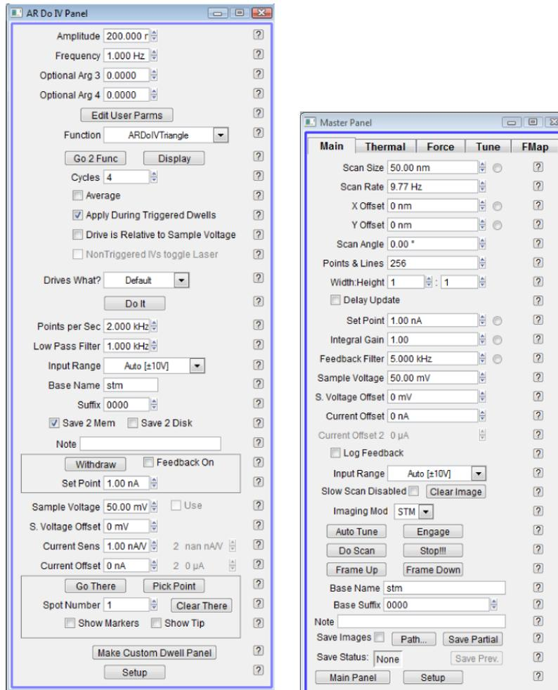
(a) DO IV Panel with highlights for STM (b) Master Panel Main Tab set up for STM imaging
