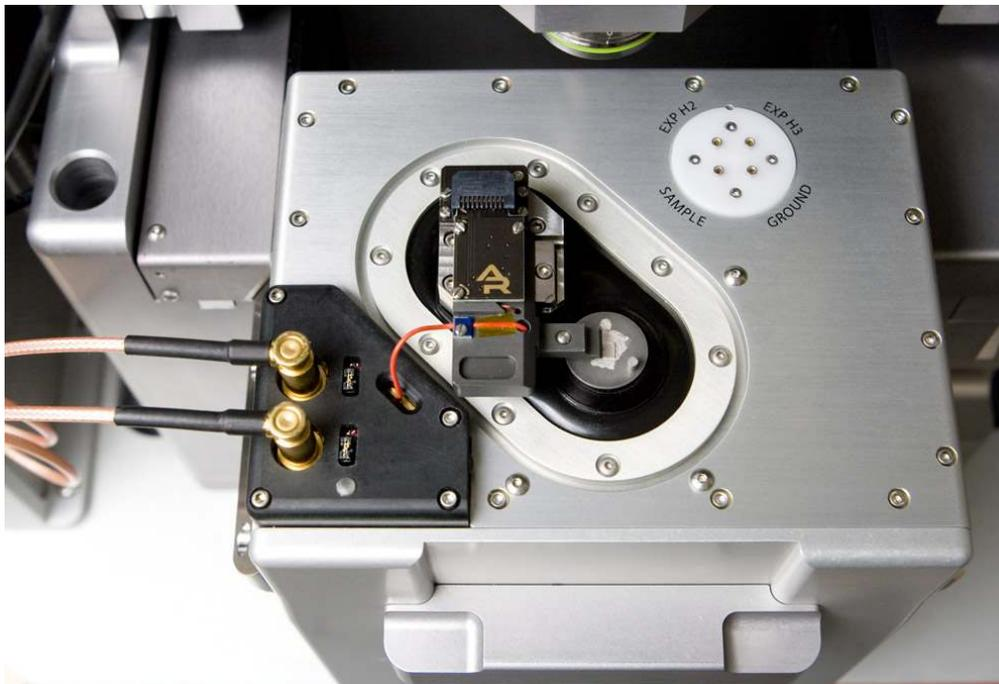
**Figure 3.2.:** Detailed view of the high voltage option.
