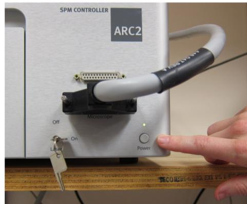
2. Double check that the laser key on the ARC2 controller is in the ON position. The red LED labeled “laser” at the front of the Cypher enclosure should be illuminated.
