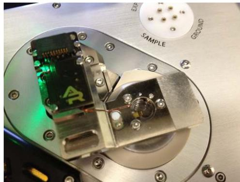
2. Push the scanner into the chassis and close the scanner clamp on the chassis.
