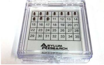
A photograph of a clear plastic tray containing 35 small, black, rectangular conductive levers. The tray is labeled with numbers 11 through 35 and the "ASYLUM RESEARCH" logo.                                 |
