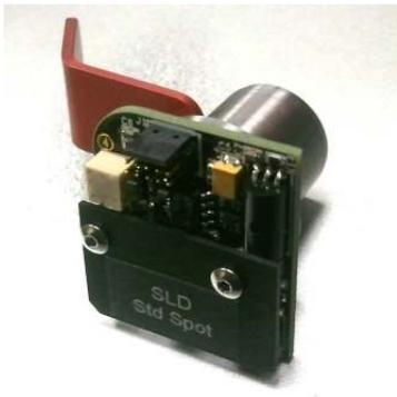
A photograph of a Super Luminescent Diode (SLD) assembly. It consists of a black printed circuit board (PCB) with a red plastic cover on top. The PCB has a silver cylindrical component on the right side. The text 'SLD Std Spot' is printed on the front of the board.                |
