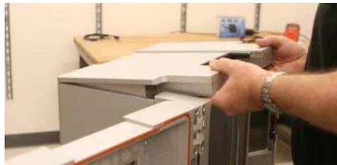
3. When the roof is on completely, shut the door on the right side carefully.
