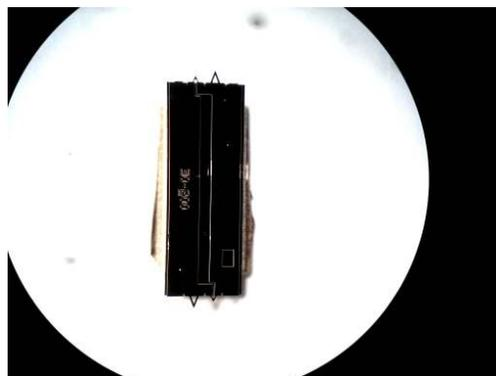
**Install an iDrive cantilever into the droplet holder**
