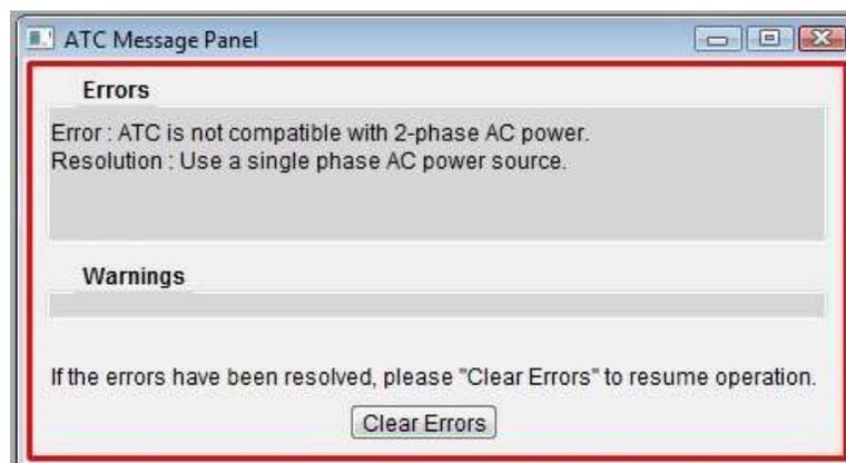
This error is caused by faulty wiring in the wall receptacle.
