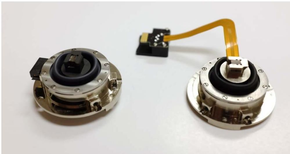
**Figure 13.6.:** Ambient stage / fluid cell body combination on the left. Heater stage / gas cell body combination on the right.
