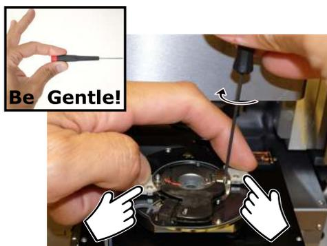
**Slide scanner into chassis:**
