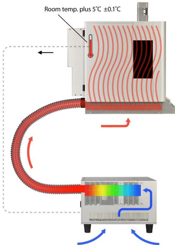
**Figure 19.1.:** Basic Diagram of ATC airflow. Cool lab air enters via a HEPA filter at the bottom of the Cypher ATC and then passes through fans and heater coils and travels via corrugated hose to the Cypher enclosure. Temperature signals travel from the Cypher back to the ATC (dotted line). Air exits the Cypher from the bottom rear.
