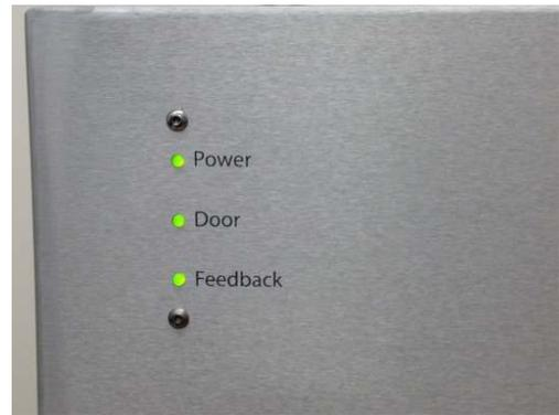
**Feedback ON, but door open:** The ATC is on, the door is OPEN and the ATC feedback loop is in Standby mode.
