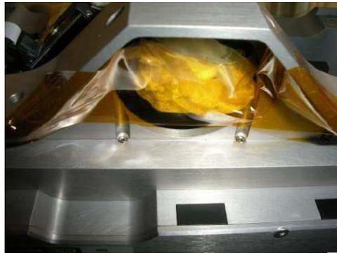
7. a) Tape down the scanner release lever
