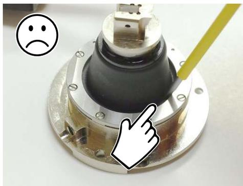
**Be careful when reattaching the cantilever clip to not crack the glass.**
