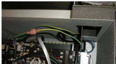
4. Next, put your hand inside the chassis and release the pass through the board from the chassis by popping it out away from the chassis.
