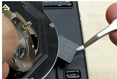
**Guide the heater cable under the ring:**
