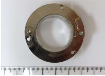
A circular, metallic fluid cell body with a central white lens and a brass-colored outer ring. A ruler is visible at the bottom for scale. |
