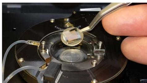
**Prepare scanner to load cantilever holder:**
