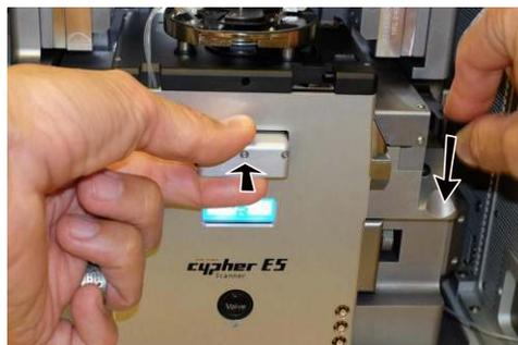
**Note** Proper seating of the scanner is most important when using the cooling capabilities of the Cooler-Heater sample stage. During normal operation it is not particularly important.
