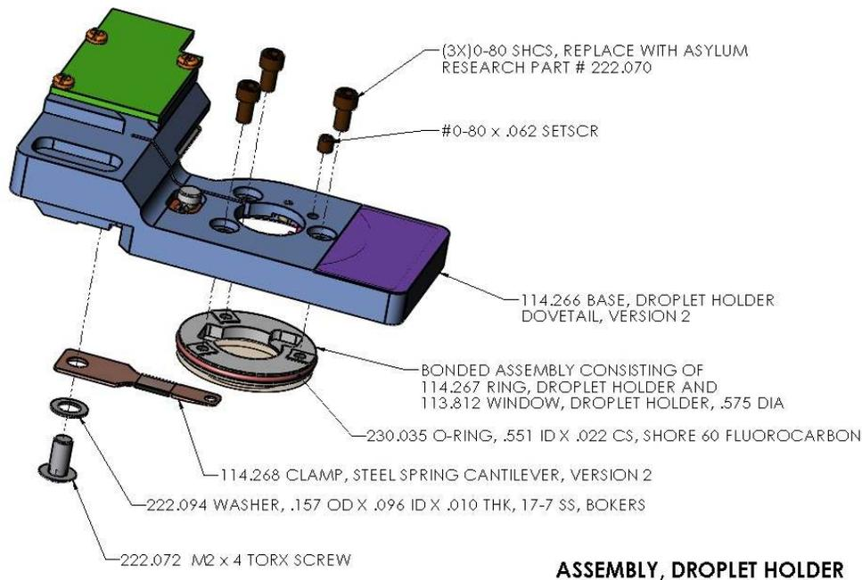
**Figure 6.3.:** Droplet Cantilever Holder Assembly Overview
