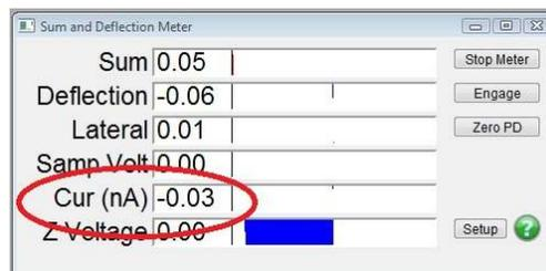
**Note** If the Sum and Deflection meter window does not update, Try adding Current as one of the data channels in the Master Channel panel and then reselect Contact mode as the imaging mode the system.
