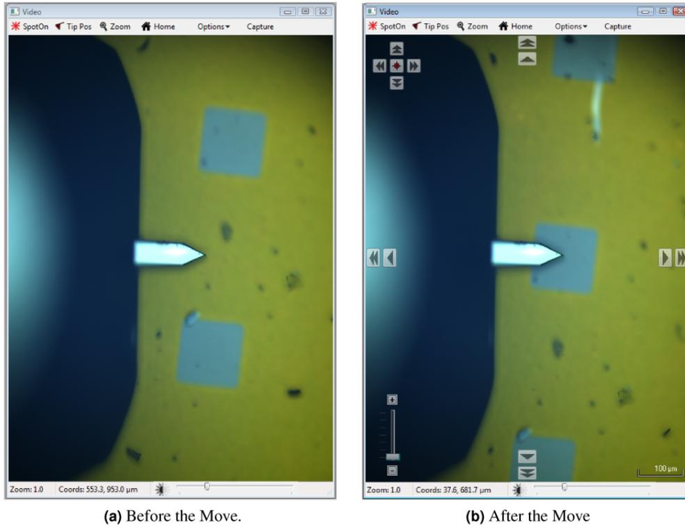
Figure 4.5.: Moving a Sample After a Scan
