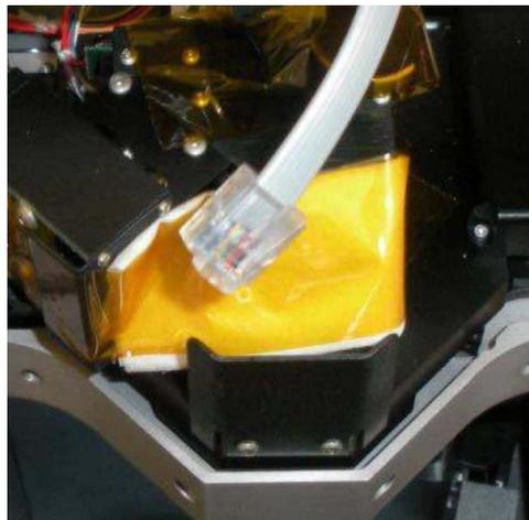
5. Kapton tape the ground cable (green & yellow cable on back side of chassis) straight down behind the board (Do not tape to the side, as it must be back to be safe from the shipping guard/mullet).
