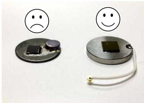
**Warning:** Pay attention! Attempting to starting a tip approach on a “non-flat” sample may cause serious damage to your cantilever holder and/or sample stage.
