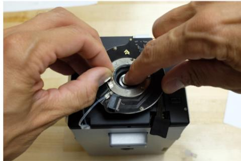
**Note** A properly seated sample stage is centered in the cell body and
