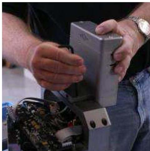
4. Set down the view module, then set aside the 2 screws and the L-key tool.
