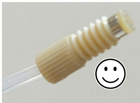
**When unlocking the sample stage from the scanner you only need 3 turns.**
