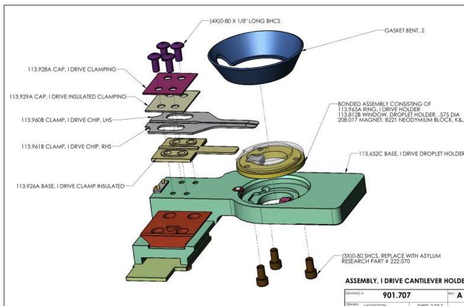
**Figure 7.3.:** Droplet Cantilever Holder Assembly Overview
