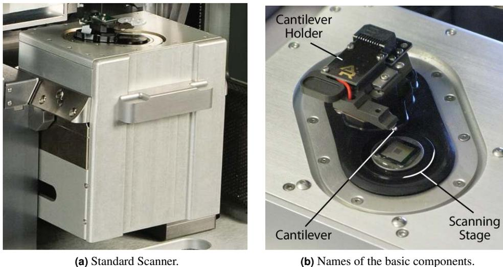
**Figure 3.1.:** The Standard Scanner
