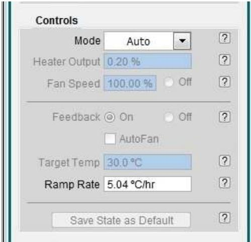
During operation, the ATC feedback will be maintained as long as the power to the ARC2 controller and ATC unit are left on. Exiting the software will not interrupt the ATC operation.
