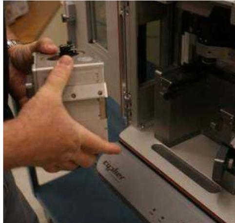
2. Remove any cantilever holders from scanner stage and set them aside.
