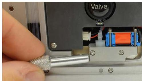
**Remove the fitting using the tool:**
