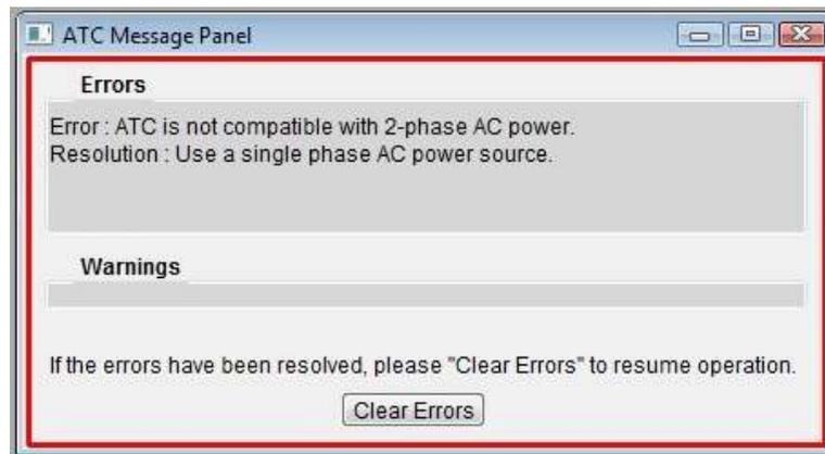
The ATC requires single phase power. This error is typically caused by the wrong type of wall power or:
