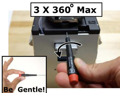
**Loosen the cell body screws:**
