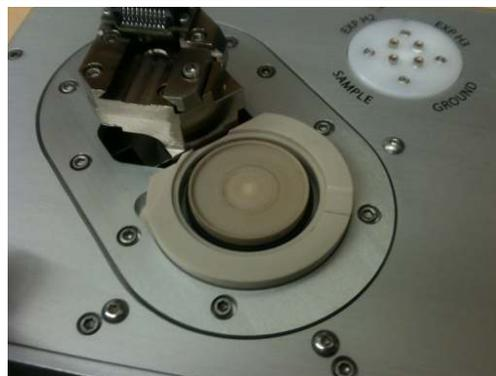
2. **Install the evaporation shield**
