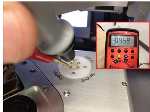
**Enter the amount of offset voltage needed in the S. Voltage Offset control parameter.**
