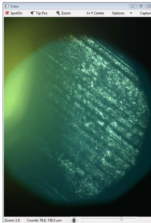
6. If you have raised the objective focus all the way up to the level of the cantilever then lower the objective back down to focus on the field diaphragm and set the sample focus there. You will be approximately 30 $\mu\text{m}$  higher than the actual sample. The result of this is a slightly longer time for the system to engage the tip.
