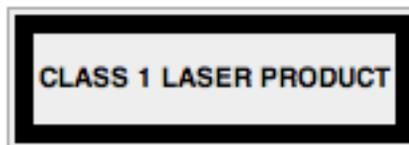
**Figure 20.2.:** A class 1 laser product (IEC 60825-1:2007 and EN60825-1:2007) is safe under all conditions of normal use.
