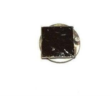
A photograph of a small, dark, square-shaped HOPG sample mounted on a circular metal disc.                                                                                                                    |
