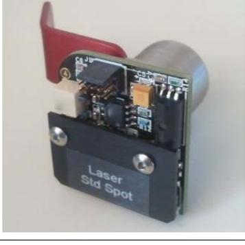
A photograph of a Laser Diode assembly with a standard spot size. It features a black PCB, a red plastic cover, and a silver cylindrical component. The text 'Laser Std Spot' is printed on the front of the board.                                                                    |
