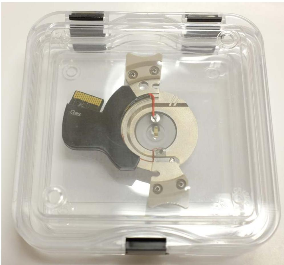
**Figure 12.1.:** A cantilever holder properly stored in its box.
