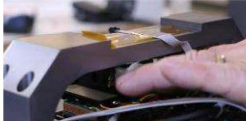
4. Put lens tissue and Kapton tape over the hot mirror and wrap tape around to cover the side port hole.
