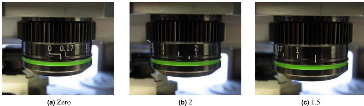
Figure 17.1.: Some examples of correction collar settings.
