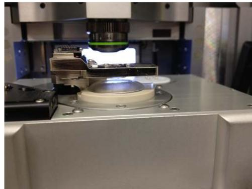
5. Secure the droplet holder to the engage pillar by tightening the dovetail clamp. Remember to only hold the driver tool with your fingertips and gently tighten the screw.
