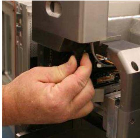
3. Unscrew and remove 2 screws from the top bridge of the view module using the 3/16" Ball End Allen Wrench L-Key. (part#290.105)-BE CAREFUL TO HOLD VIEW MODULE TIGHTLY WITH YOUR OTHER HAND BECAUSE IT WILL FALL FORWARD OTHERWISE!!!
