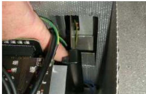
5. Once released, slowly pull the backpack toward yourself, carefully guiding both the disconnected pass through the board and the ground cable through the hole so as to separate it completely from the chassis.
