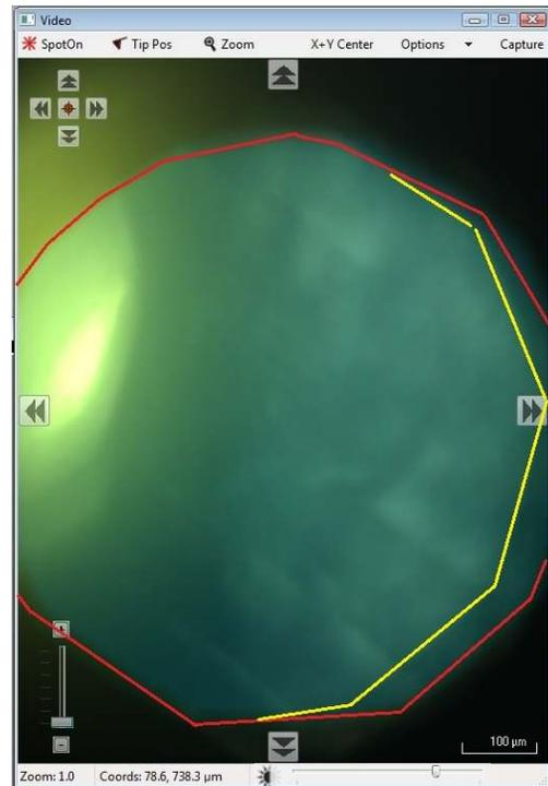
4. One way to confirm this is to note the focus position distance located just below the arrow buttons. Raise the objective back up to focus on the field diaphragm and note how much the focus distance has changed. Typically, the sample focus distance is about  $30\mu\text{m}$  below the focus distance of the field diaphragm.
