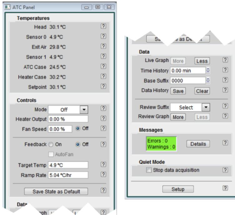
Figure 19.2.: Typical View of the ATC control panel.
