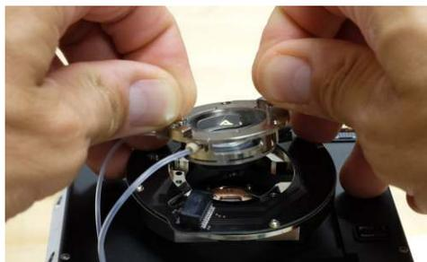
**Loosen fittings of gas in/out lines:** In this step, you will remove the gas in/out lines. Notice that the gas lines are sealed by a small O-ring which may or may not come out when you pull out the gas lines.
