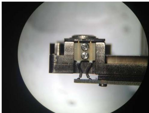
**Tip** Aligning the cantilever clip on the body
