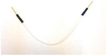
A photograph of a white, flexible bias wire assembly with two black electrical connectors at the ends.                                                                                                       |
