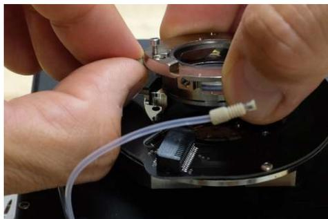
5. Check the gas lines to see if small O-rings are stuck to the end. Usually the rings will stay inside the cell, but in case they are stuck to the gas lines, please unstuck them and place aside.
