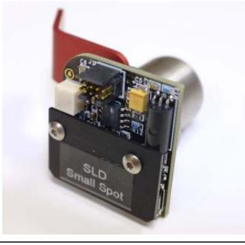
A photograph of a Super Luminescent Diode (SLD) assembly with a small spot size. It is similar in design to the standard spot size assembly, with a black PCB, a red plastic cover, and a silver cylindrical component. The text 'SLD Small Spot' is printed on the front of the board. |
