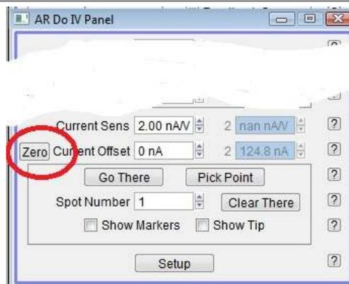
**Press the 'Zero' button to zero the current**
