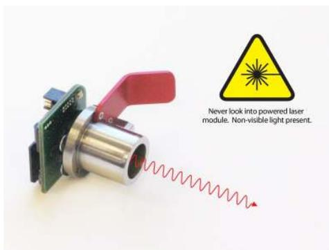
**Figure 20.4.:** Light source module removed from the Cypher AFM. During the removal process it is possible to tamper with safety overrides in such a way that collimated light shines out of the module. As a safety precaution, never look directly into the module while its power cable is attached (power cable not shown in this image).
