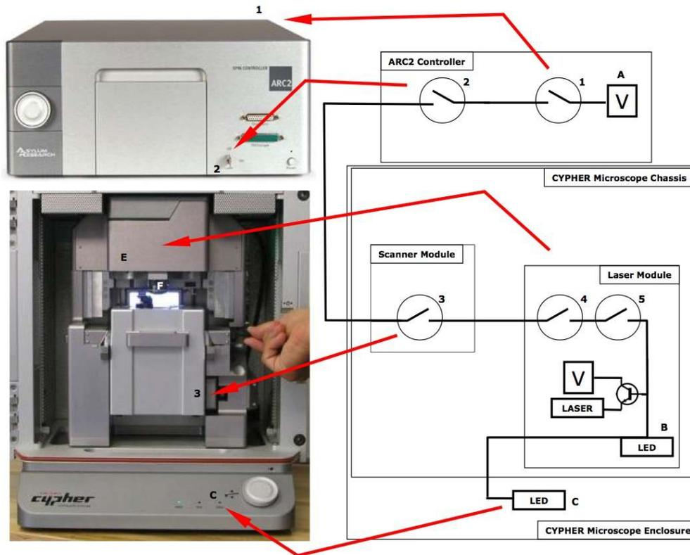
**Figure 20.5.:** Cypher and ARC2 laser safety interlock system. (A) Laser Voltage Source. (1) Back panel remote interlock connector, or Light Source Remote Jack. (2) Front panel laser power key switch. (3) Scanner interlock. (4,5) Laser module dual magnetic switch interlock. (B) Laser Module LED. (C) Cypher enclosure laser LED. (E) Optical system cover. (F) Objective Lens. Not shown is an additional software controlled laser power switch.
