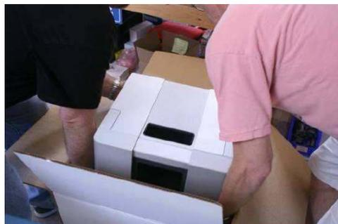
15. Place 1-2 plastic bags over the enclosure once it is already in the box to protect the finish from damage.
