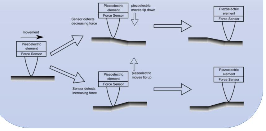
The sharp probe, feedback mechanism, highprecision piezoelectric scanner, and optical lever Piezoelectric Scanner
